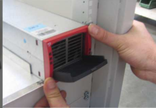
(2) Push firmly till the connection is properly engaged
